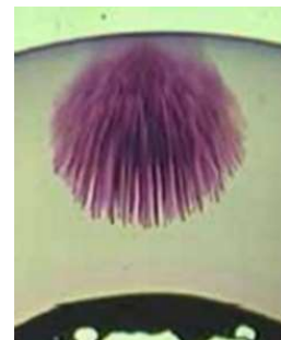
Figure 5: Localized Water Tree growth.
